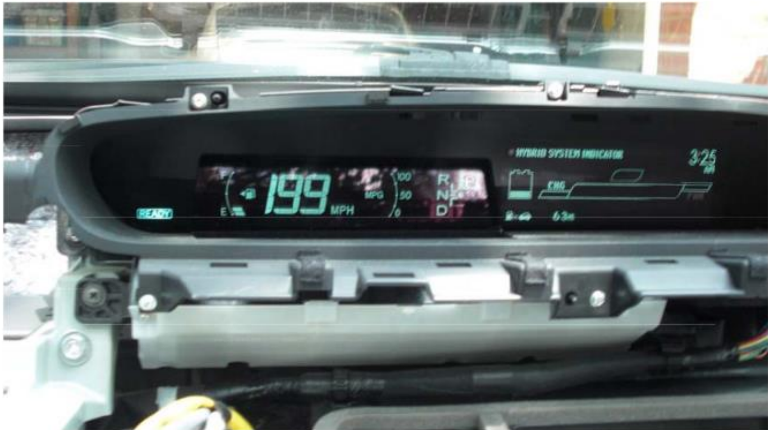
Figure 17: The speedometer can be altered to display any value.
