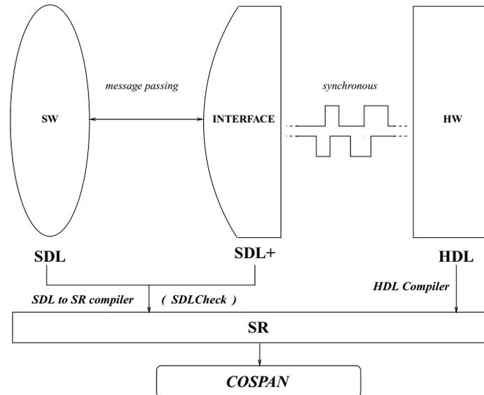
Figure 4. The general structure of the tool support.
