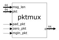
The packet "multiplexer", *pktmux*, provides the current packet to be stored in the register file. Because there are 4 types of packets (see slide 11), *pktmux* has 3, mutually-exclusive control inputs:
