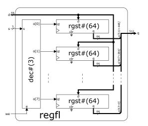
The dec#(3) is an instance of the dec module available parameterized with the value of 3 for the selection line's width.
