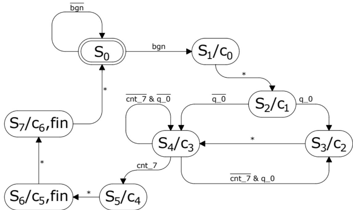
**Important:** Control unit must be triggered by the opposite edge of the clock, compared to all the other sequential elements in the architecture!
